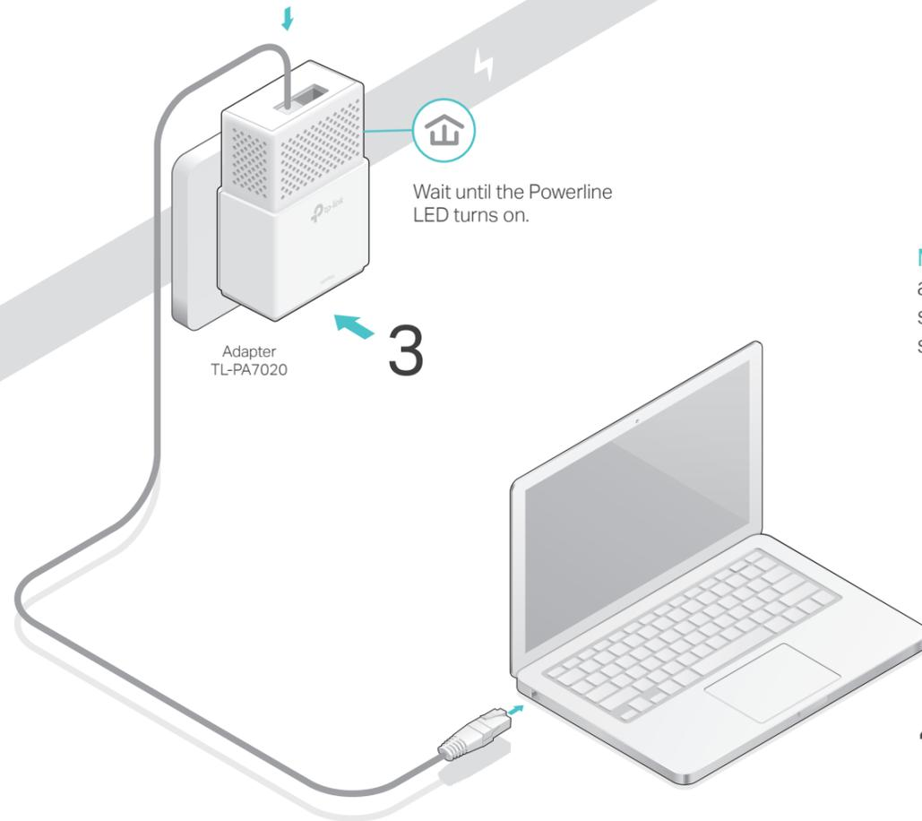
**More:** To add additional Powerline adapters and extenders with the default settings, simply plug them into the wall sockets on the same electrical circuit.
