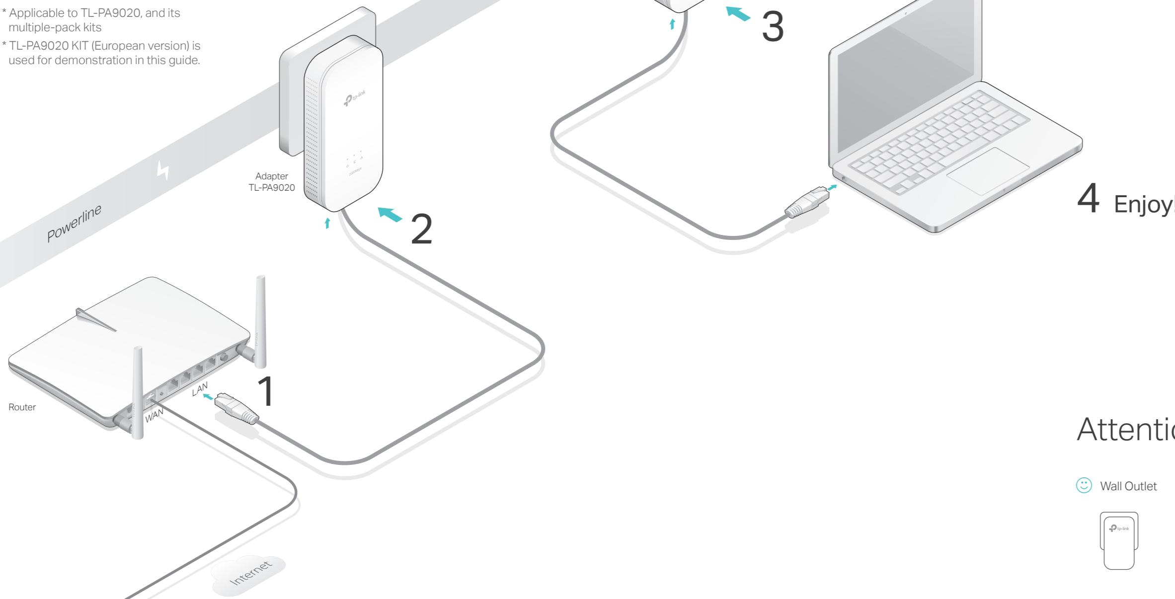
**More:** To add additional powerline adapters and extenders with the default settings, simply plug them into the wall sockets on the same electrical circuit.
