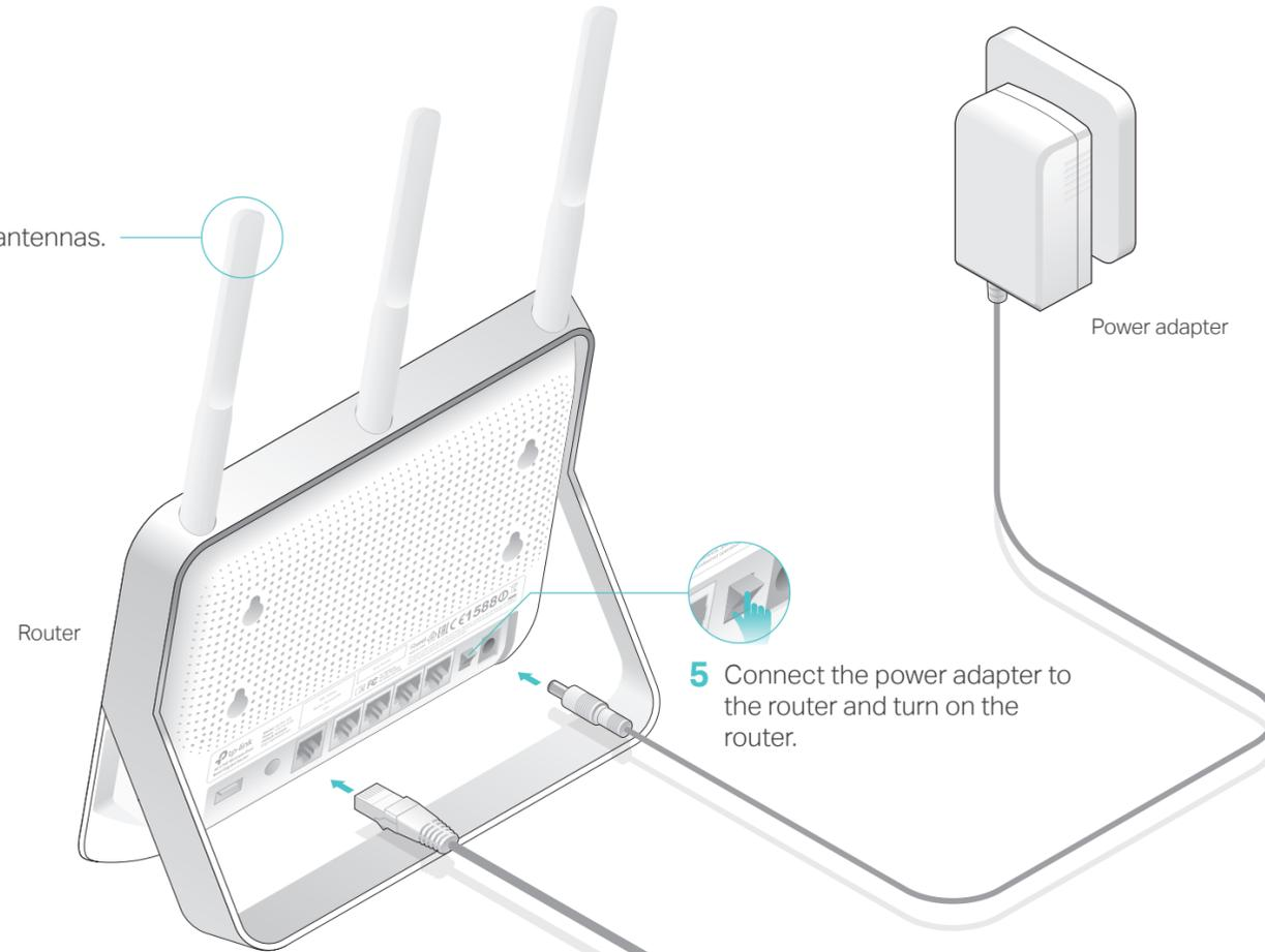
**5** Connect the power adapter to the router and turn on the router.
