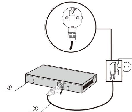
① Switch (Rear Panel)      ② AC Power Cord (with PE cable)
