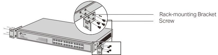
3. After the brackets are attached to the device, use suitable screws (not provided) to secure the brackets to the rack, as illustrated in the following figure.
