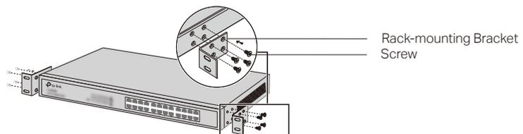
3. After the brackets are attached to the device, use suitable screws (not provided) to secure the brackets to the rack, as illustrated in the following figure.
