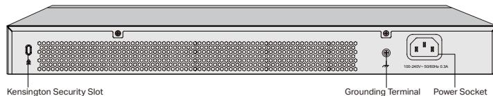
The rear panel of T1500-28PCT is shown as the following figure.
