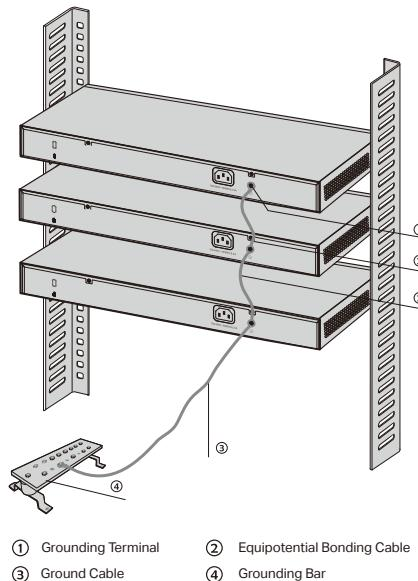
When equipotential bonding, please note that the cable should be copper wrapped Kelly with its area being  $6mm^2$  at least. The shorter cable the better, and use a grounding bar to establish an equipotential bonding point.
