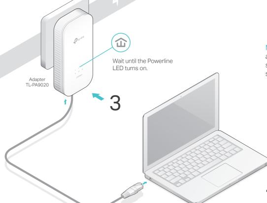
More: To add additional powerline adapters and extenders with the default settings, simply plug them into the wall sockets on the same electrical circuit.
