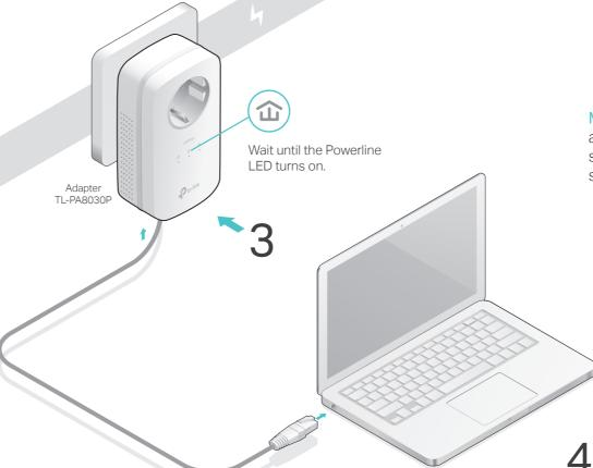
More: To add additional Powerline adapters and extenders with the default settings, simply plug them into the wall sockets on the same electrical circuit.
