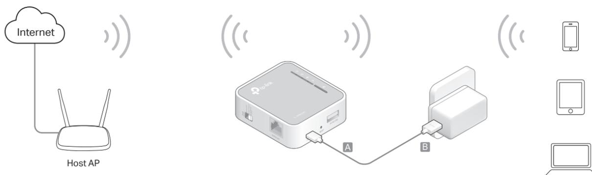
1. Switch the operation mode to **AP/Rng Ext/Client** and plug the router's adapter into an electrical outlet near your host AP.
