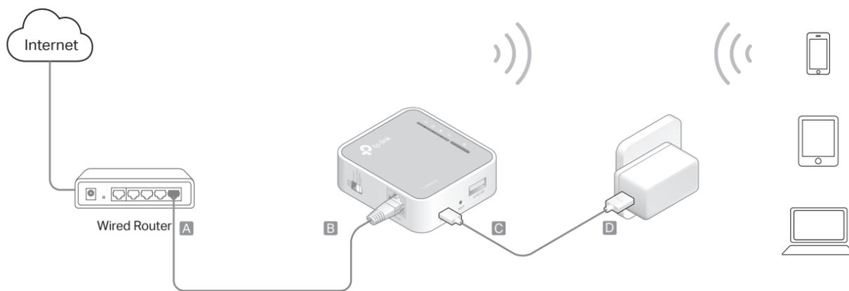
1. Switch the operation mode to **AP/Rng Ext/Client** and connect the hardware according to Step A to D in the left diagram.
