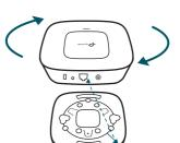
Attach the EAP to the mounting bracket by aligning the arrow mark ▼ on the EAP with the arrow mark \ on the mounting bracket, then rotate the EAP until it locks into place, as shown on the left.
