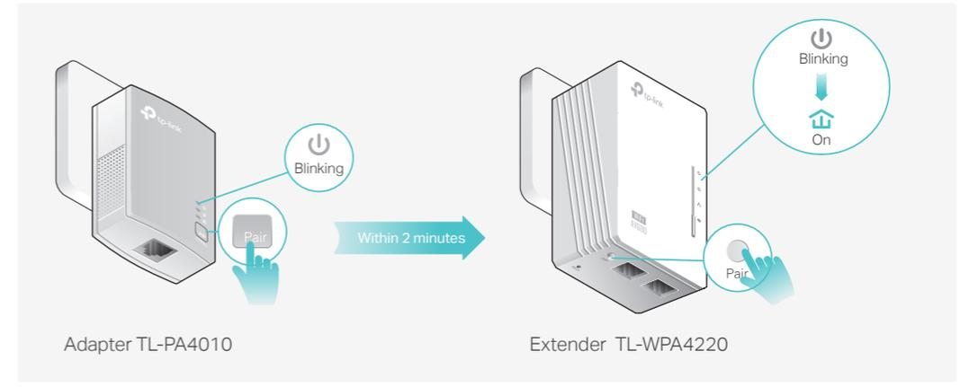
**4** Pair Adapter and Extender B by referring to step 3. Extender B will automatically sync Wi-Fi settings from Extender A.
