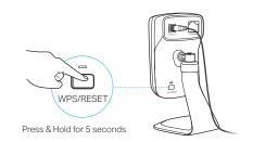
While the camera is powered on, press the WPS/RESET button for 5 seconds until the System LED on the front panel goes off. The camera will reset and reboot.
