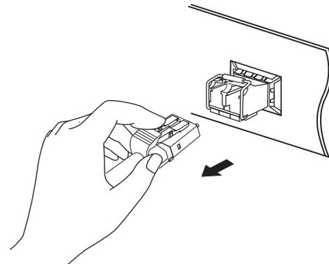
3. Pull the safety latch downwards to release the SFP, and then pull it out from the slot.
