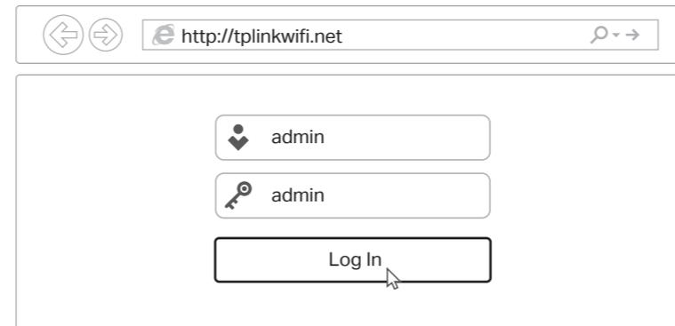
**B** Run the **Quick Setup**, choose the **Wireless Router** operation mode, then follow the instructions to complete the initial configuration.
