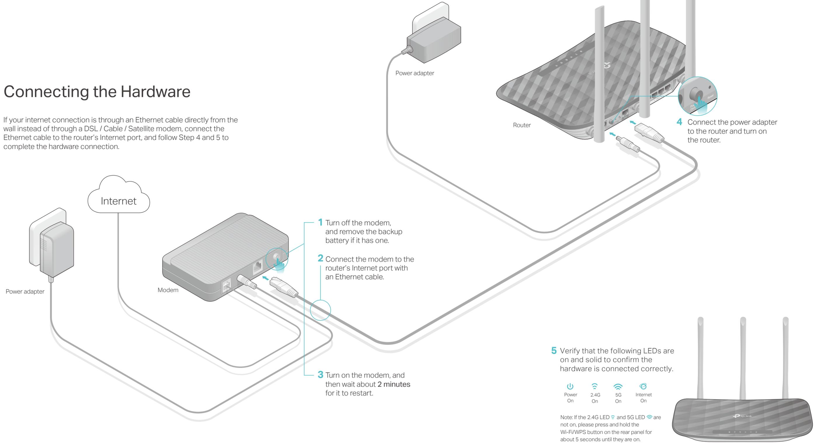
**1** Turn off the modem, and remove the backup battery if it has one.
