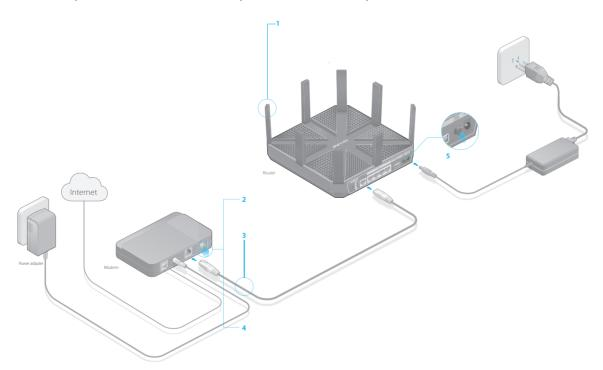
1) Place the router horizontally and extend the antennas to the maximum angle.
