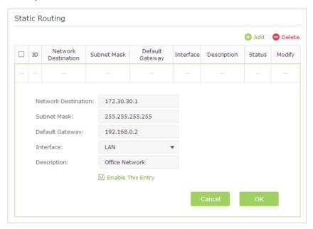
Network Destination: The destination IP address that you want to assign to a static route. This IP address cannot be on the same subnet with the WAN IP or LAN IP of the router. In the example, the IP address of the company network is the destination IP address, so here enters 172.30.30.1.
