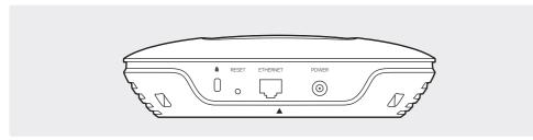
With the device powered on, press and hold the button for about 8 seconds until the LED flashes red, then release the button. The device will restore to factory default settings.
