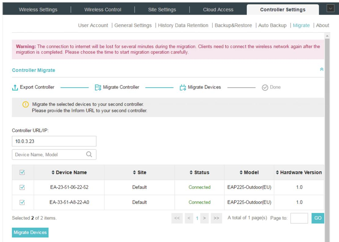
**Note:** Make sure that TCP/UDP ports 29810–29813 is enabled on the computer, so the EAPs can communicate with the controller via the ports. If the firewall and antivirus software block these ports, they also block the packets between the controller and EAPs.
