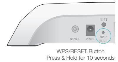
A2. Log in to the web management page of the modem router, and go to Maintenance > SysRestart, select Factory Default Settings and click RESTART, then wait until the reset process is complete.
