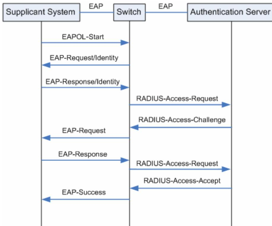
Figure 11-18 EAP-MD5 Authentication Procedure
