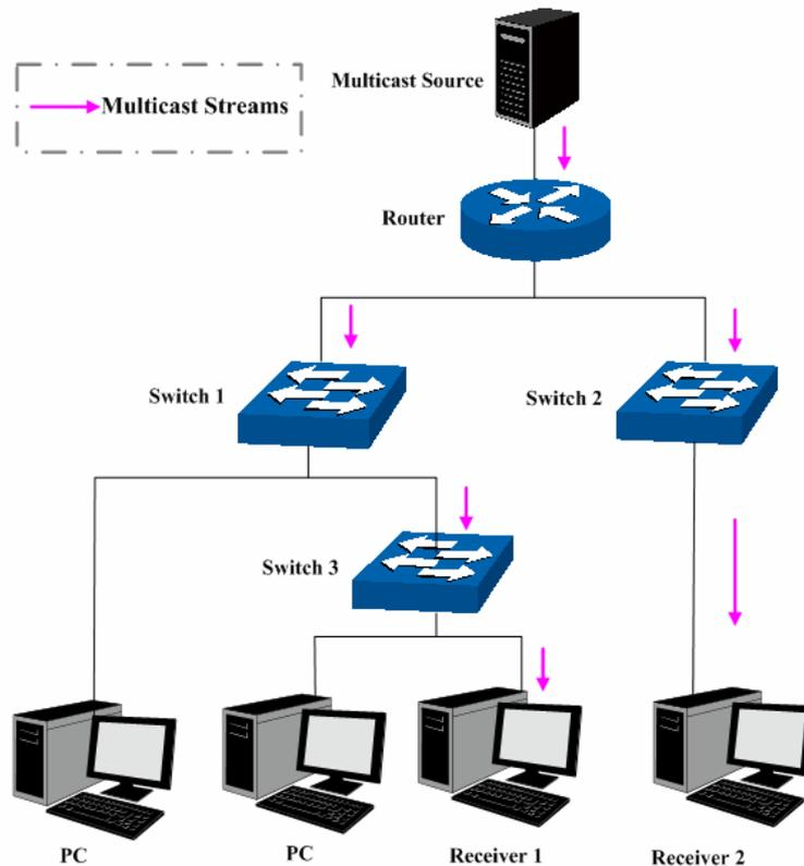
Figure 8-1 Information transmission in the multicast mode
