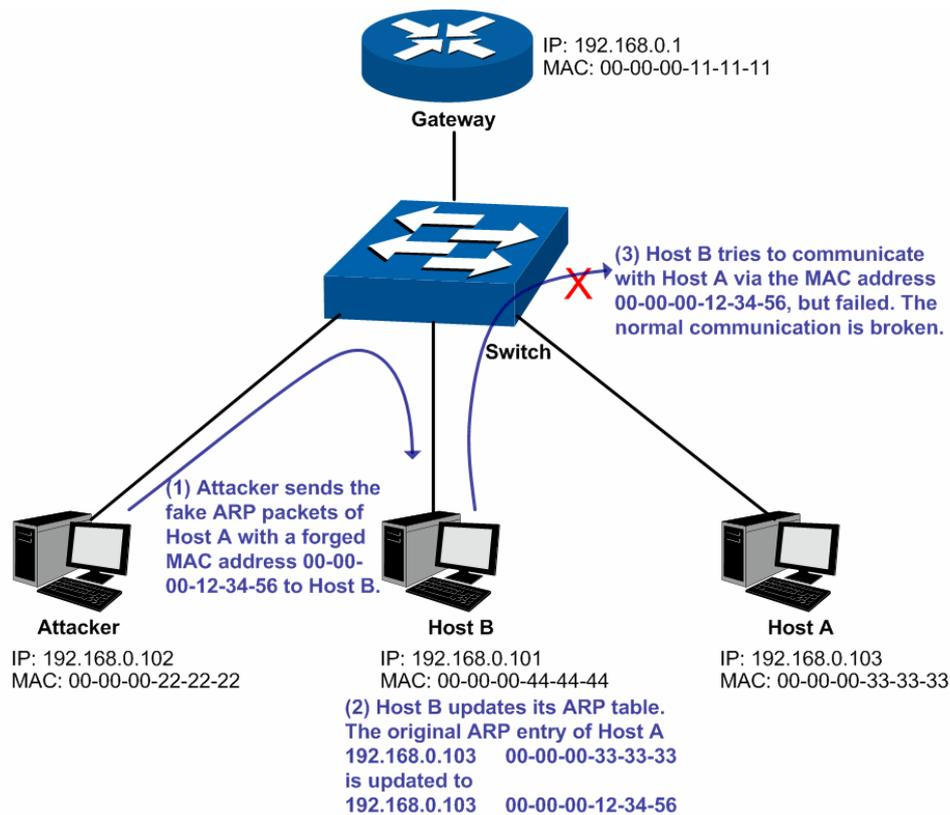
Figure 11-11 ARP Attack – Cheating Terminal Hosts
