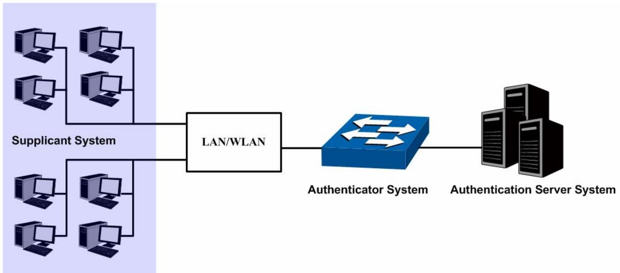
Figure 11-17 Architecture of 802.1X authentication
