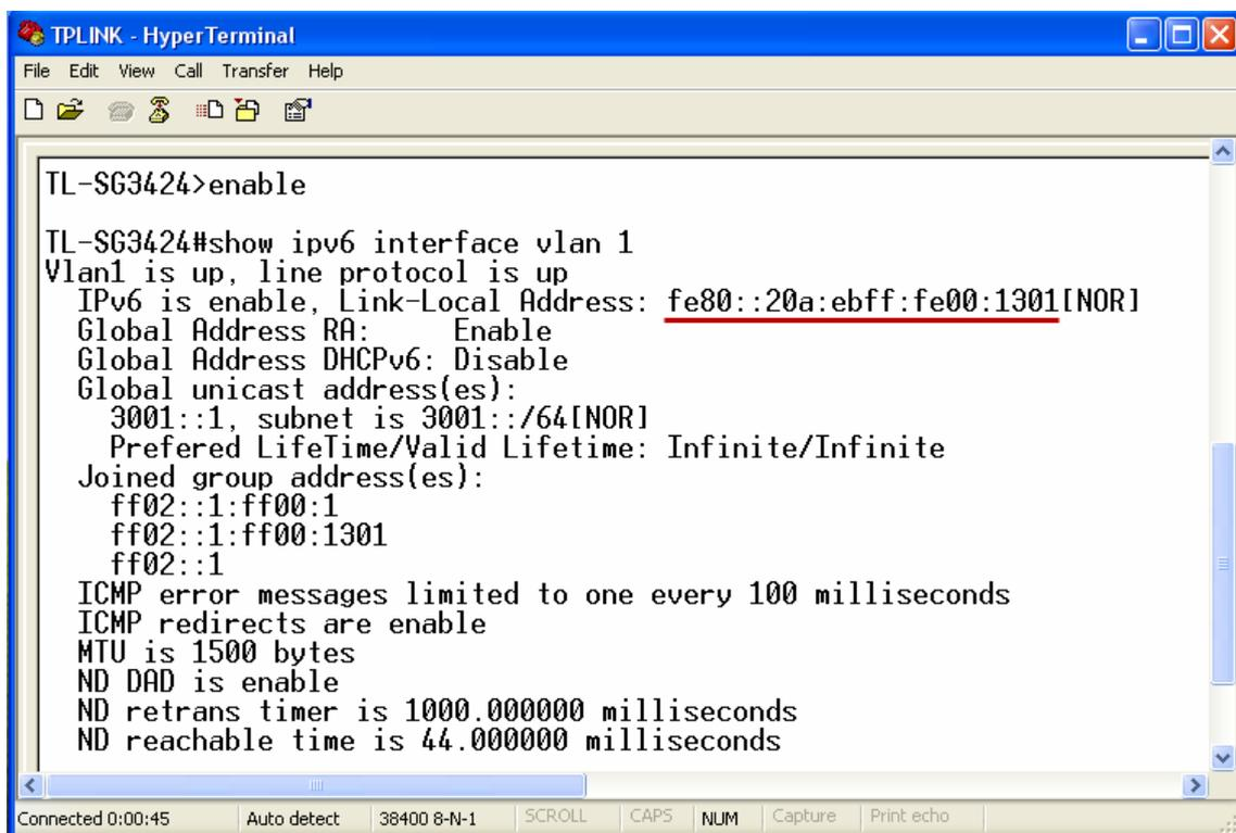
Figure 3-4 The Switch's Link-local Address
