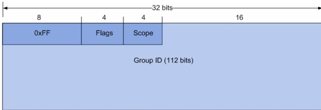
0XFF at the start of the address identifies the address as being a multicast address.
