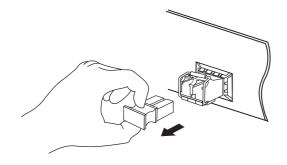
4. Plug a fiber-optic cable into the SFP. Note that the SFP works without any additional configuration.
