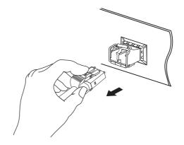
3. Pull the safety latch downwards to release the SFP, and then pull it out from the slot.
