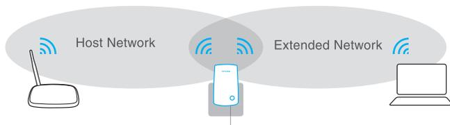
② Wait until the (Signal Strength) LEDs are lit. Make sure the extender is in a location with **3 or more LEDs lit**. If not, **relocate it closer to the router** to achieve a good (or better) signal quality.
