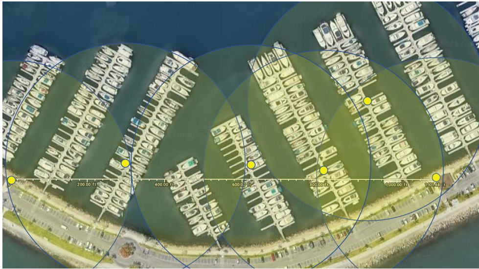
A yacht club wireless deployment example with EAP225-Outdoor
