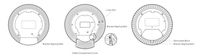
**Note:** For an AP with a Cable Compartment Cover, to avoid device damage, do not insert any objects into the holes for attaching the cover!
