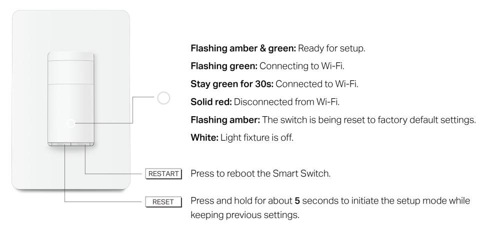
Press and hold for about **10** seconds to factory reset the switch.
