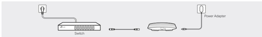
Plug one end of the provided power adapter into the POWER port of the EAP and the other end to a standard electrical wall outlet.
