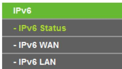
There are three submenus under the IPv6 Support menu: **IPv6 Status**, **IPv6 WAN** and **IPv6 LAN**. Click either of them, and you will be able to scan or configure the corresponding function. The detailed explanations for each submenu are provided below.
