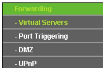
There are four submenus under the Forwarding menu: **Virtual Servers**, **Port Triggering**, **DMZ** and **UPnP**. Click any of them, and you will be able to configure the corresponding function.
