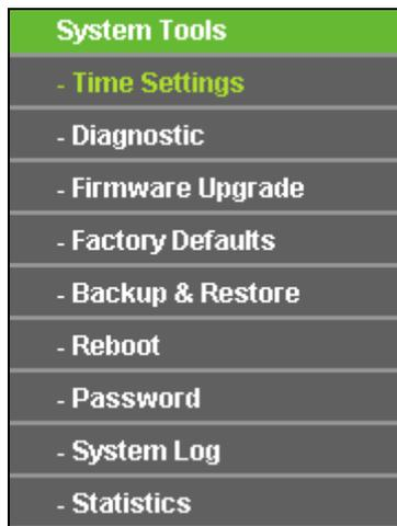
Choose menu “**System Tools**”, and you can see the submenus under the main menu: **Time Settings**, **Diagnostic**, **Firmware Upgrade**, **Factory Defaults**, **Backup & Restore**, **Reboot**, **Password**, **System Log** and **Statistics**. Click any of them, and you will be able to configure the corresponding functions. The detailed explanations for each submenu are provided below.
