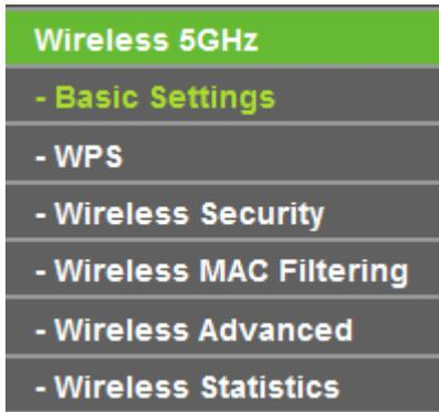
There are six submenus under the Wireless menu: **Basic Settings**, **WPS**, **Wireless Security**, **Wireless MAC Filtering**, **Wireless Advanced** and **Wireless Statistics**. Click any of them, and you will be able to configure the corresponding functions.
