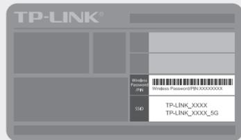
b Click the network icon of your computer or go to Wi-Fi Setting of your smart device, and then select the SSID to join the network.
