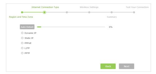
5. In this case, the router automatically detects Dynamic IP as the connection type. Click Next.
