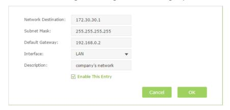
Network Destination: The destination IP address that you want to assign to a static route. This IP address cannot be on the same subnet with the WAN IP or LAN IP of the router. In the example, the IP address of the company network is the destination IP
