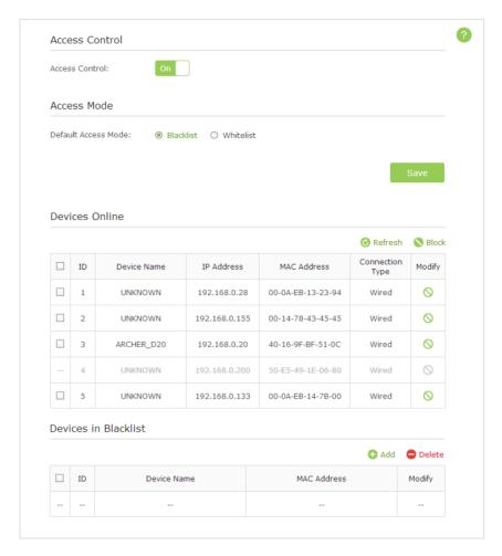
**4.** Select the access mode to either block (recommended) or allow the device(s) in the list.
