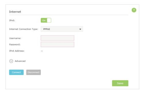
4) 6to4 Tunnel: An IPv4 Internet connection type is a prerequisite for this connection type. (4. 2) Click Advanced to have more configuration if ISP requires. Click Save to save the settings and then click Connect to finish the configuration.
