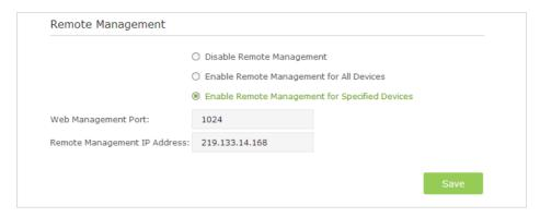
Devices using this WAN IP can manage the router by logging in to http://Router's WAN IP:port number (such as http://113.116.60.229:1024).
