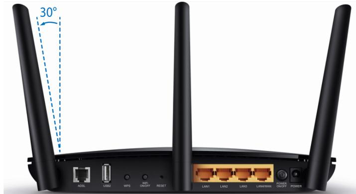
The modem router's back panel shows the antennas, connection ports and buttons. Refer to the following for detailed instructions.
