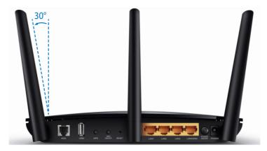
The modem router's back panel shows the antennas, connection ports and buttons. Refer to the following for detailed instructions.
