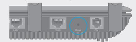
Reset Button Press & Hold for 8 seconds
