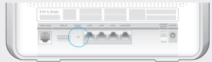
RESET Button Press & Hold for 8 seconds
