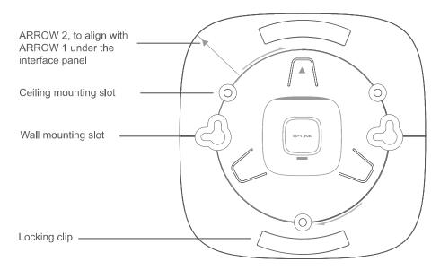
Figure 2-3 Structure of the Mounting Bracket
