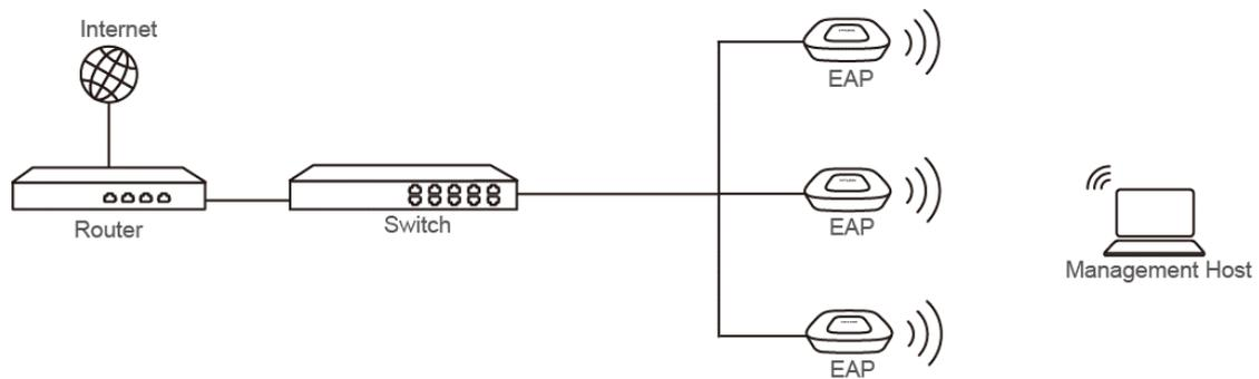
Figure 4-1 Sample Network Diagram for Wireless Login
