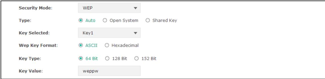
The screenshot shows a configuration form for WEP security mode. The fields are: Security Mode (WEP), Type (Auto, Open System, Shared Key), Key Selected (Key1), Wep Key Format (ASCII, Hexadecimal), Key Type (64 Bit, 128 Bit, 152 Bit), and Key Value (weppw).
