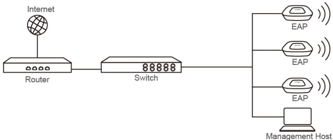
Figure 4-2 Sample Network Diagram for Wired Login
