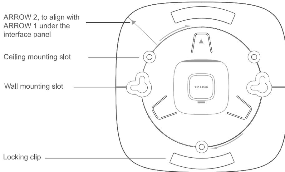
Figure 2-3 Structure of the Mounting Bracket
