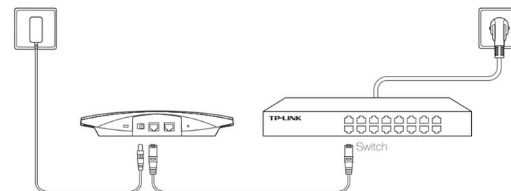
Plug one end of the provided power adapter into the POWER port of the EAP and the other end to a standard electrical wall outlet.
