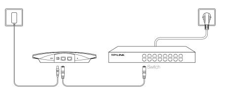
Plug one end of the provided power adapter into the POWER port of the EAP and the other end to a standard electrical wall outlet.
