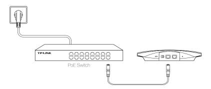
Connect the Ethernet cable from the PoE switch to the ETHERNET port.
