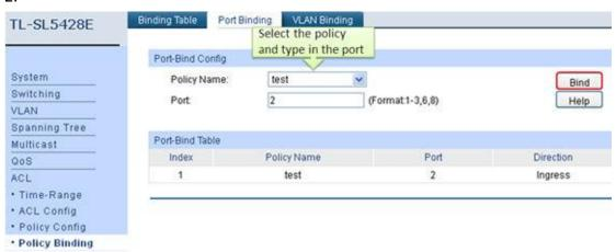
Now all configurations are completed, and the PC connected to port 2 won't get any IP address via router (DHCP server).
