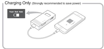
\*The M5360 can't be charged and charge the other devices at the same time.
