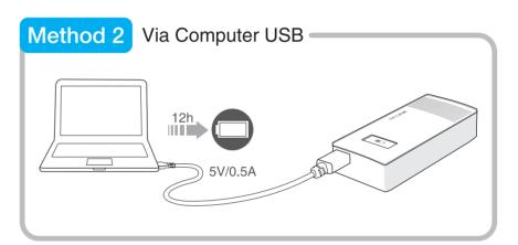
\*The M5360 has been fully charged when the lighting symbol (  $\checkmark$  ) of battery icon disappeared.
