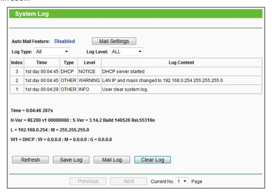
The device can keep logs of all traffic. You can query the logs to find what happened to the device.
