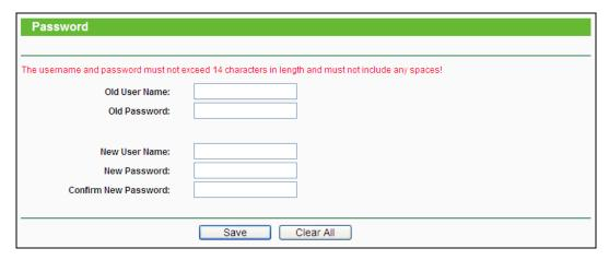
It is strongly recommended that you change the factory default user name and password of the device. All users who try to access the device's web-based management page or Quick Setup will be prompted for the device's user name and password.
