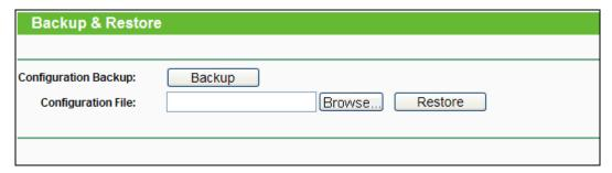
Figure 4-21 Save or Restore the Configuration
