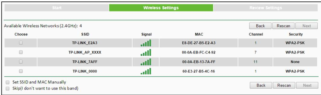
Figure 3-5 Quick Setup – Available Wireless Networks
