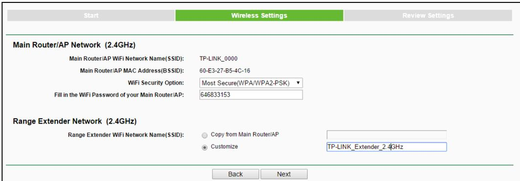
Figure 3-6 Quick Setup – Wireless Settings
