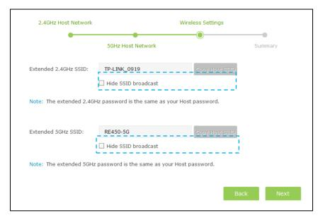
Verify your wireless settings and click Finish. The corresponding LEDs (2.4GHz and 5GHz) should turn on and stay solid.
