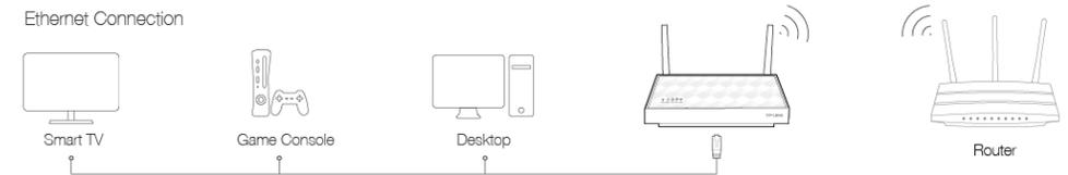
By default, the Ethernet ports connect to the 5GHz wireless network. If you want your Ethernet-enabled device to connect to the 2.4GHz host wireless network only, please follow the steps below to finish the settings:
