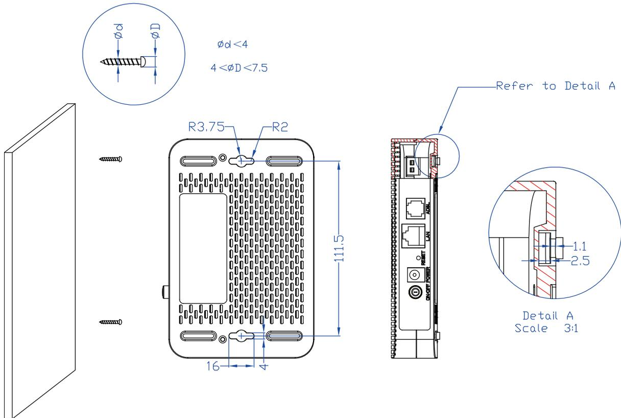
Figure 2-4 Wall-mount Install
