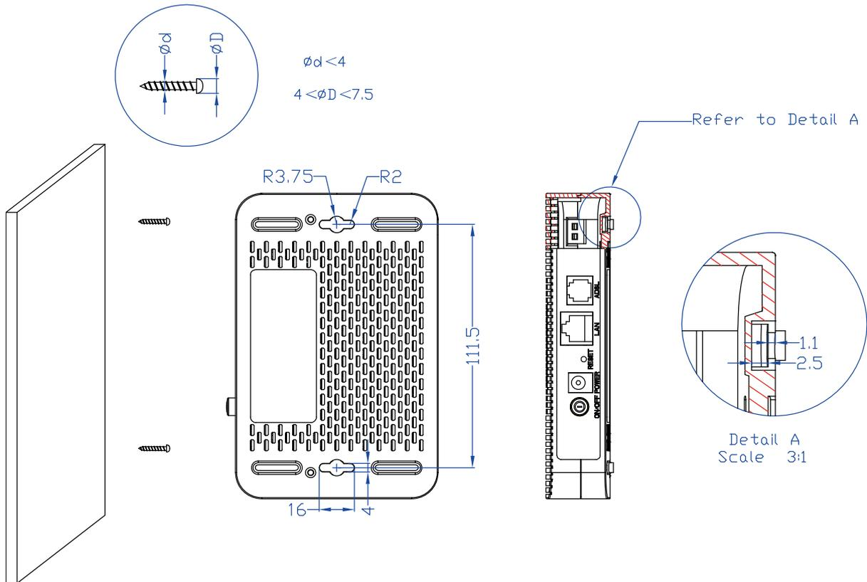
Figure 2-4 Wall-mount Install
