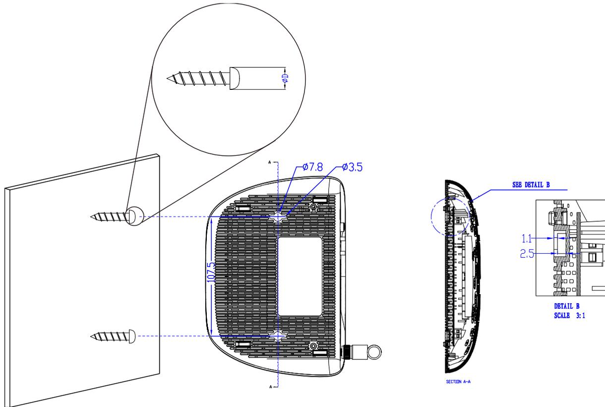
Figure 2-3 Wall-mount Install
