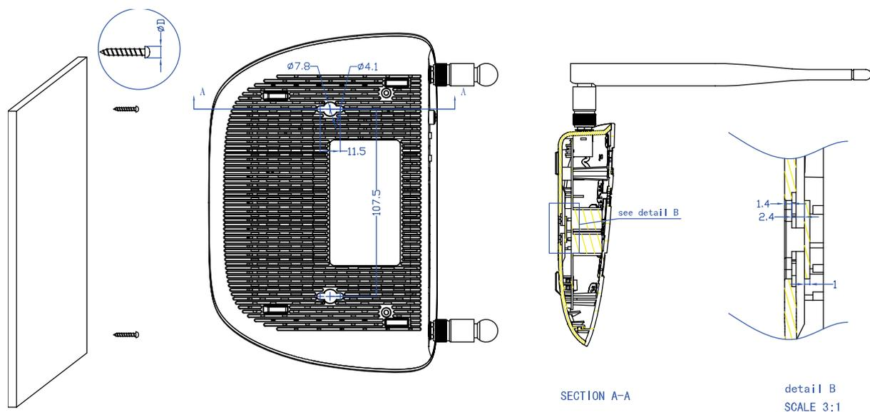
Figure 2-1 Wall-mount Install
