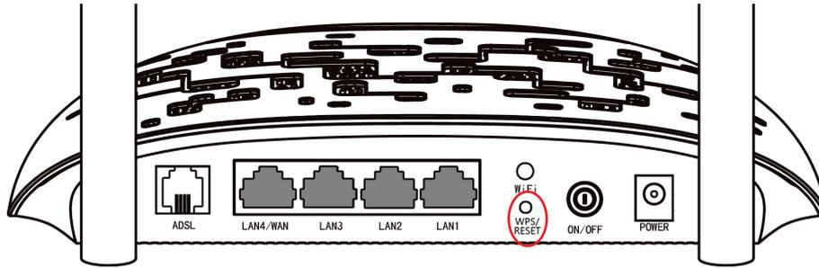
Step 2: Press and hold the WPS button of the adapter (if it has one) for 2 or 3 seconds.
