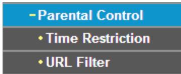
Choose “**Advanced Setup**”→“**Parental Control**”. You can configure the Parental Control function on the screen as shown in Figure 4-37. Time Restriction allows you to control the Internet activities of the children by restricting the time of surfing. URL Filter limits the computers you choose to access certain websites. These two features work independently.
