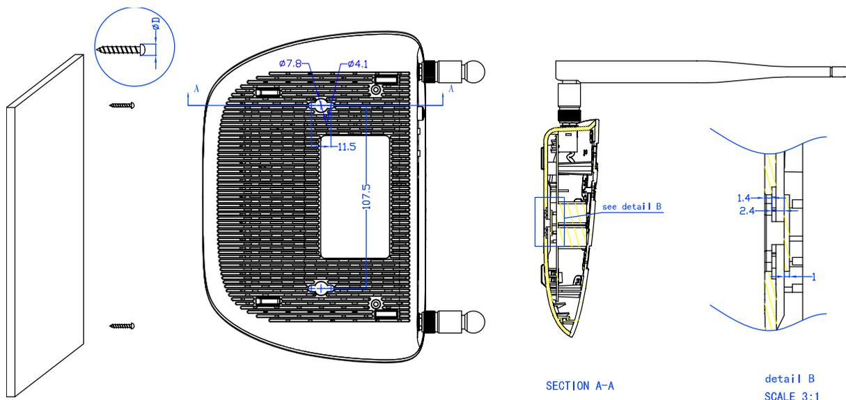
Figure 2-1 Wall-mount Install
