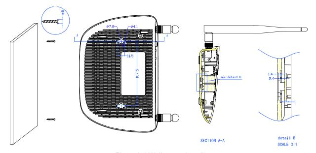
Figure 2-1 Wall-mount Install
