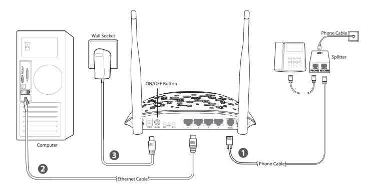
Press the **ON/OFF** button of your modem router and make sure the LEDs (especially the ADSL LED) display as shown
