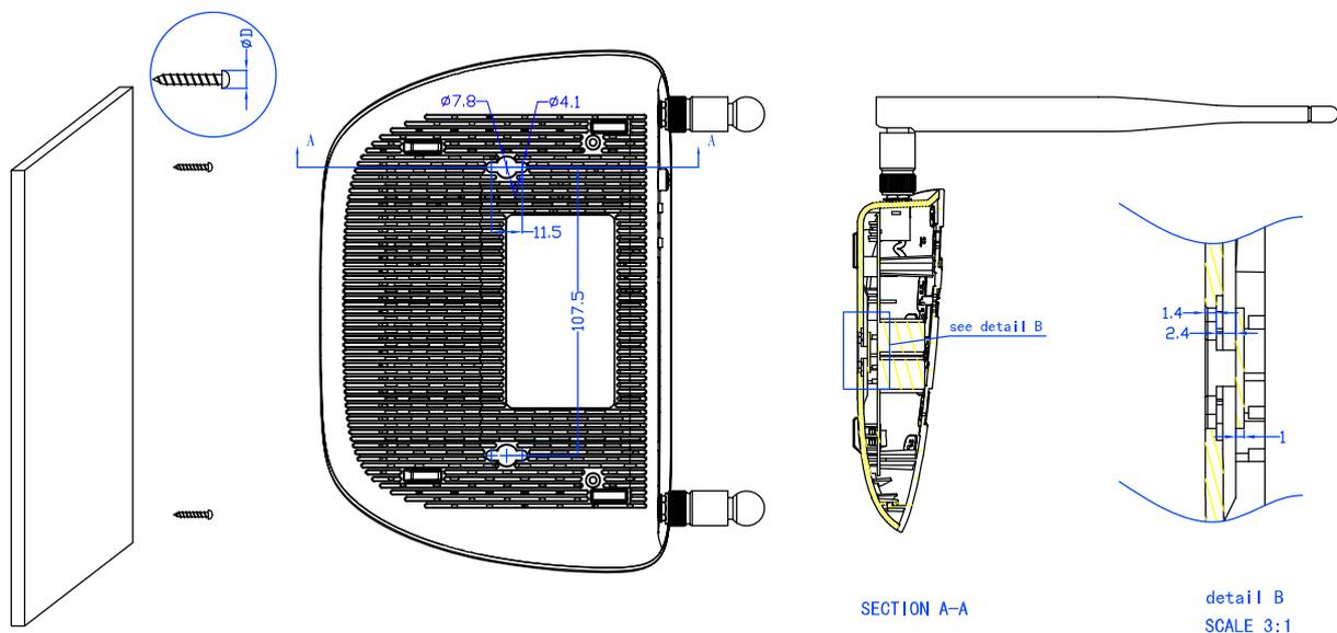
Figure 2-1 Wall-mount Install
