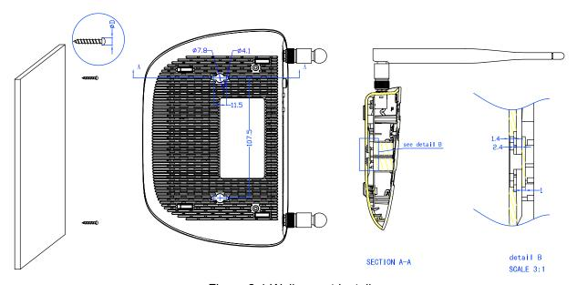
Figure 2-1 Wall-mount Install
